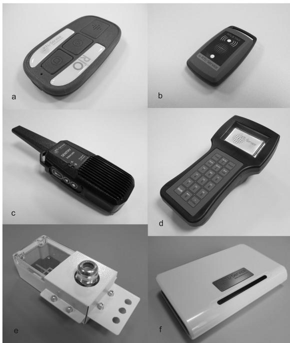
Fig. 5. RealTrac technology hardware: (a) duplex intercom Rio®; (b) tag –mobile sensor; (c) half-duplex intercom radio Sentry®; (d) wireless handheld network analyzer; (e) industrial outdoor access point; and (f) indoor access point
